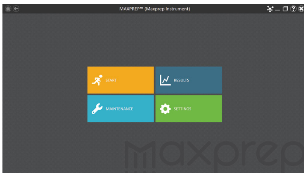
Figure 30. Maxprep™ software 'Home' screen. Selecting the Maintenance button opens the 'Maintenance' screen from which maintenance methods for the Maxprep™ Liquid Handler can be run.
